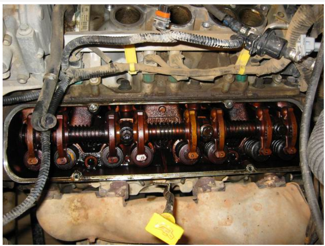
LH rocker cover and gasket removed
