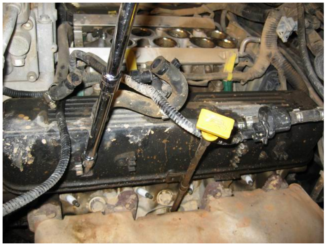
LH rocker cover and gasket removed
