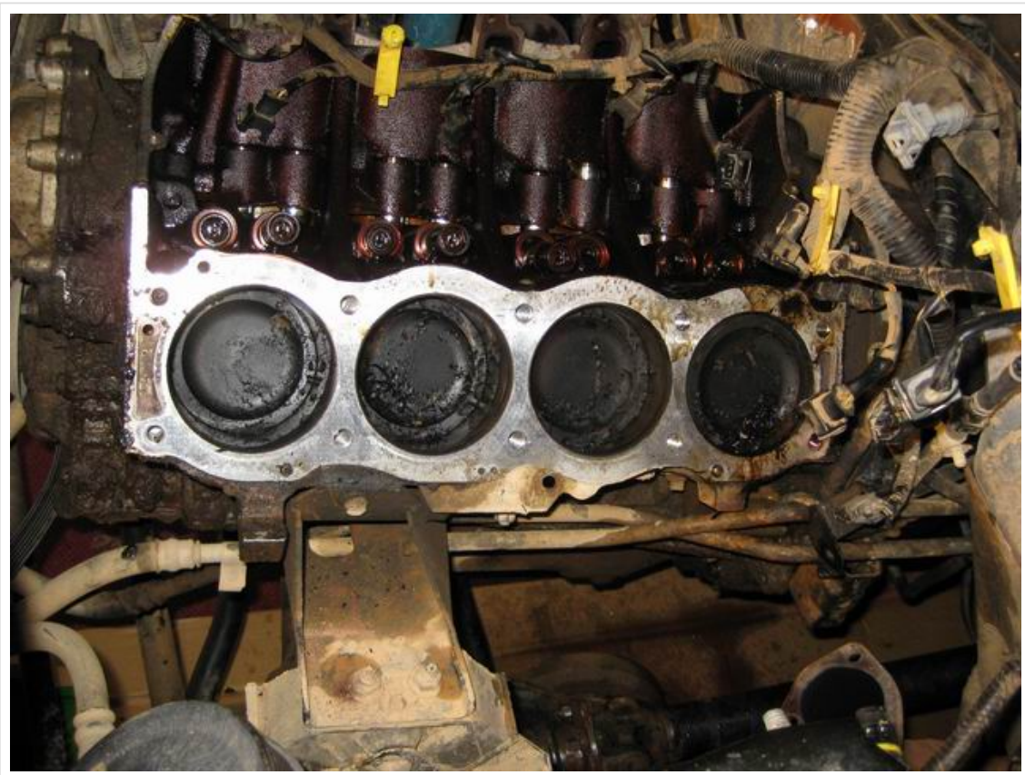
LH cylinder head removed.
