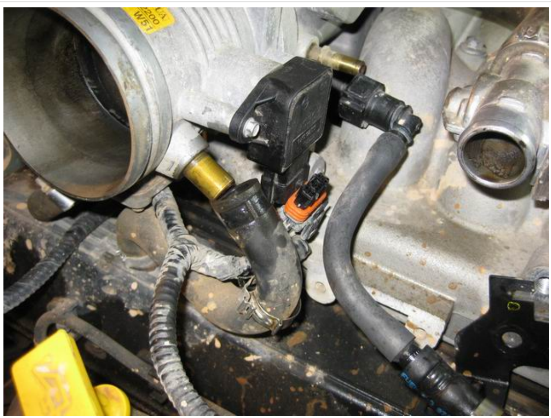
Centre – remove breather and coolant hoses from throttle body. Use a rag to soak up any coolant leakage.
