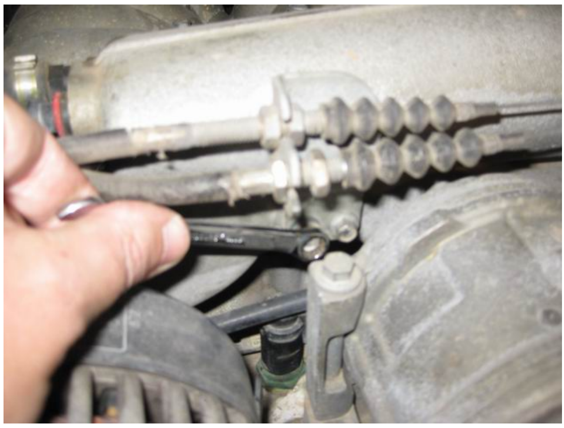
LHS – Disconnect the EVAP pipe, breather pipe, and TP sensor multiplug.
